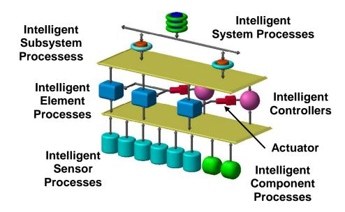
**Sensor Processes** utilize data; hence, data must be available at each intelligent sensor process. Processes within intelligent sensors must assess the quality of the data and the health of the sensor. These processes may reside in physical intelligent sensors or virtual ones (that turn legacy sensors into intelligent ones).
