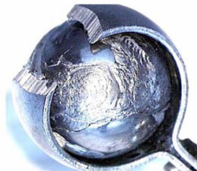
Figure 18.—Bearing grease contaminated with dirt and damage to the ball.
