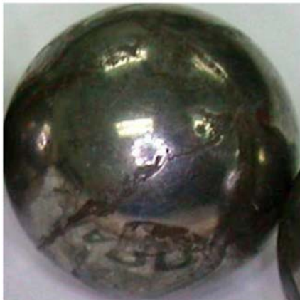
Figure 11.—Oil cooler fan bearing damage.
