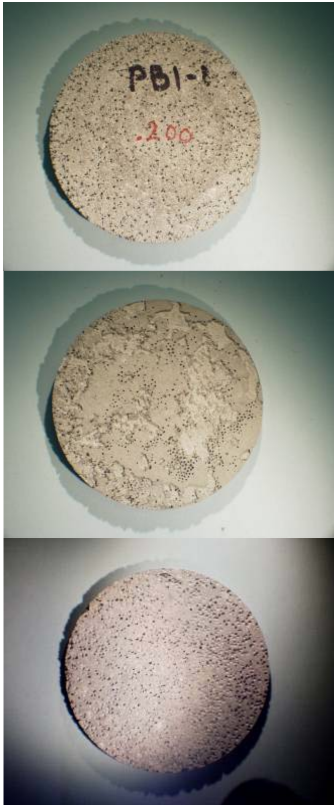
Figure 12.—Sample PB1-1 (front and back as-received; back as-sanded).
