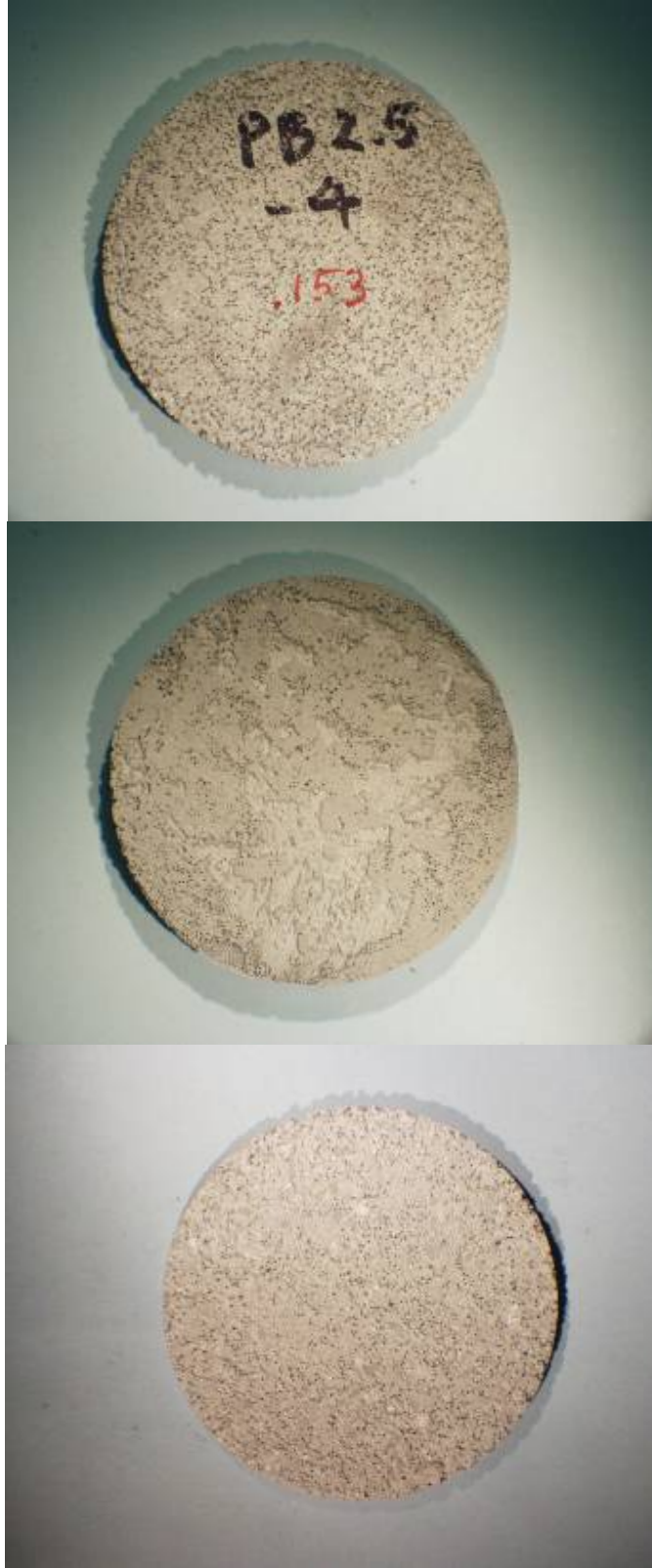
Figure 19.—Sample PB2.5-4 (front and back as-received; back as-sanded).
