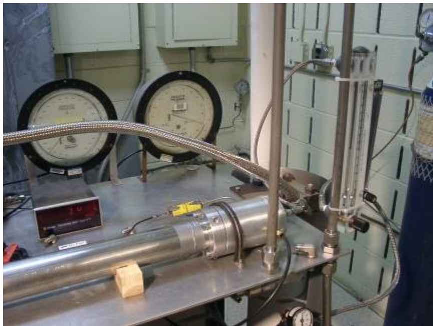
Figure 2.—Pressure gauges and flowmeter.
