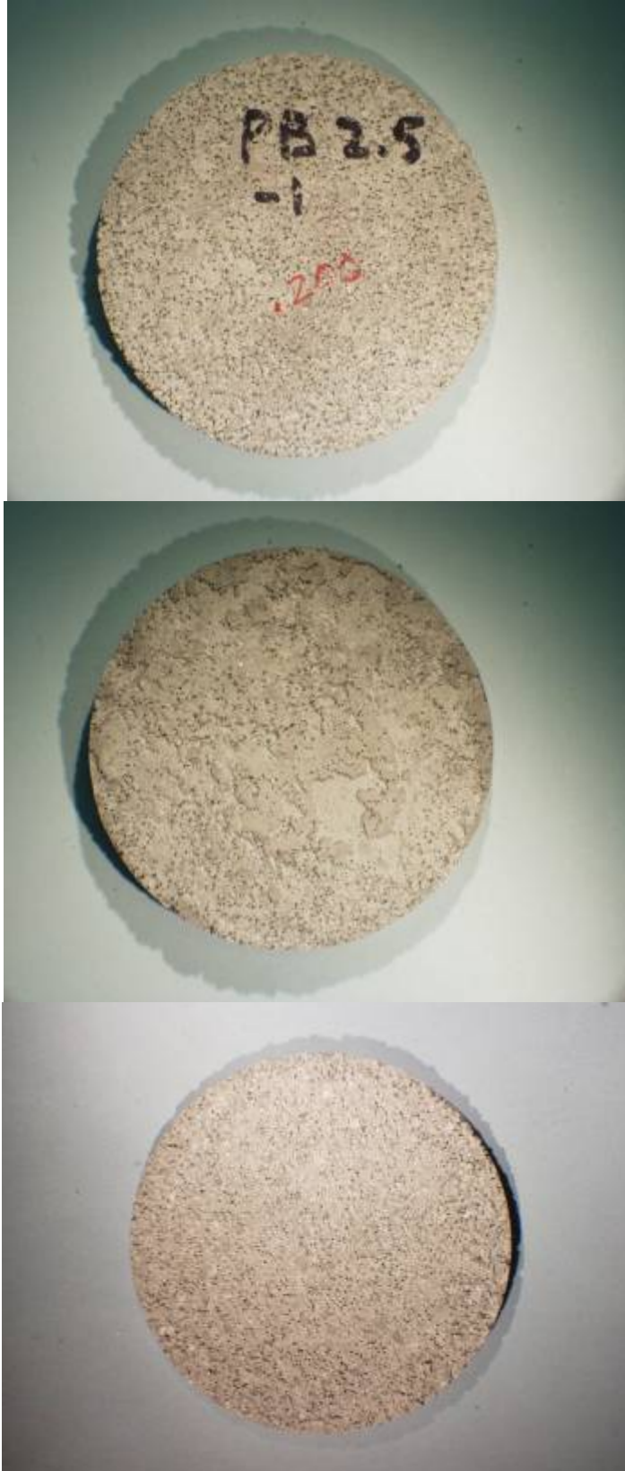
Figure 16.—Sample PB2.5-1 (front and back as-received; back as-sanded).
