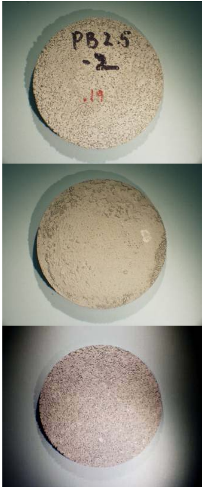
Figure 17.—Sample PB2.5-2 (front and back as-received; back as-sanded).
