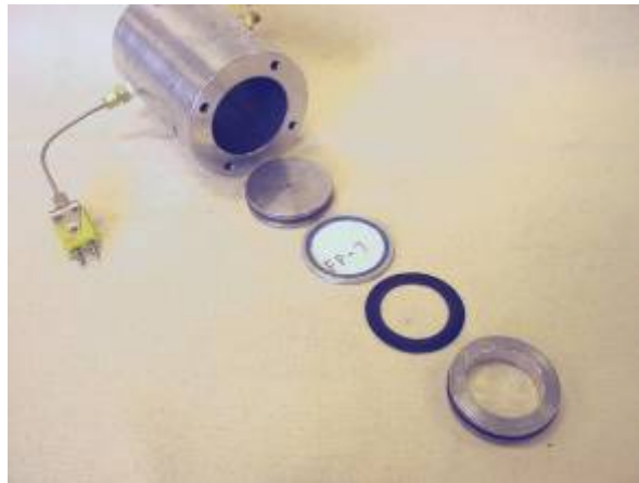
Figure 5.—Sample insertion order: flow orifice, potted sample (RTV faces upstream), gasket, downstream orifice.
