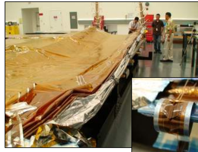
Soft Sunshield Membrane Covers Decrease Mass and Stowed Volume
