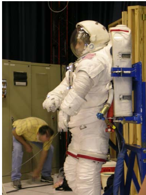
Figure 1. Photograph of a crewmember in the donning stand with the retro reflective markers on the DCM and the right hand.
