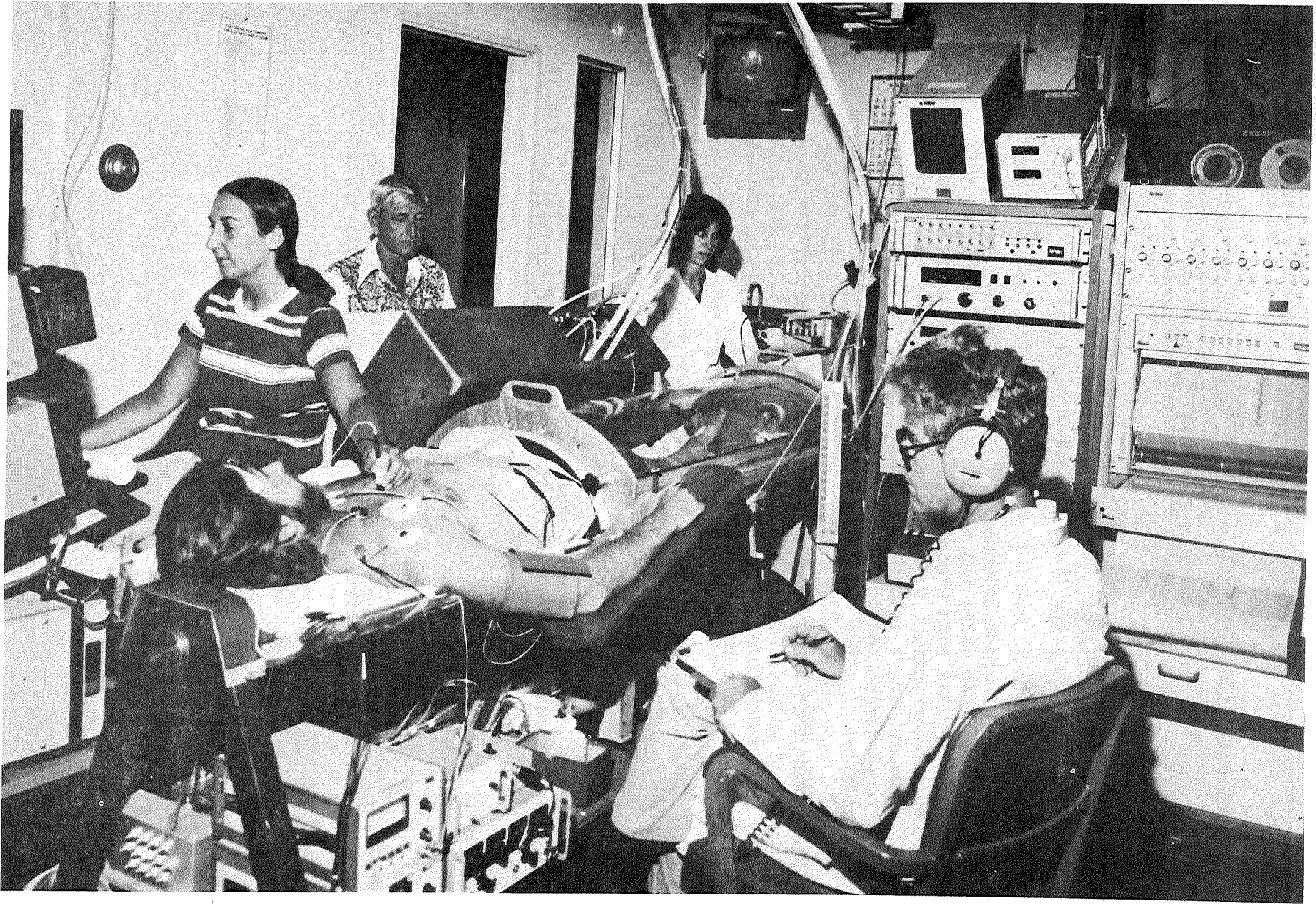
A bedrest subject undergoes LBNP. The horizontal chamber encasing the subject's lower body is evacuated to -50 mmHg. An echocardiographic technician is imaging his heart during this stress.
