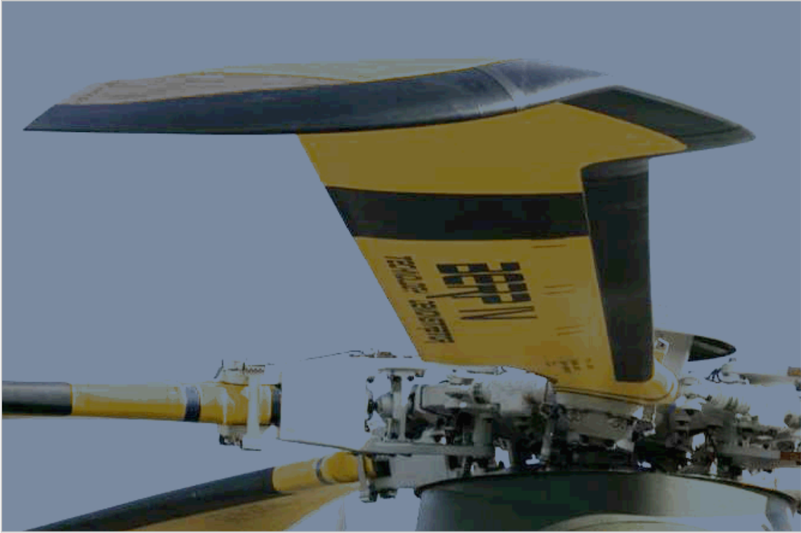
Figure 2. BERP IV blade tip design [5].
