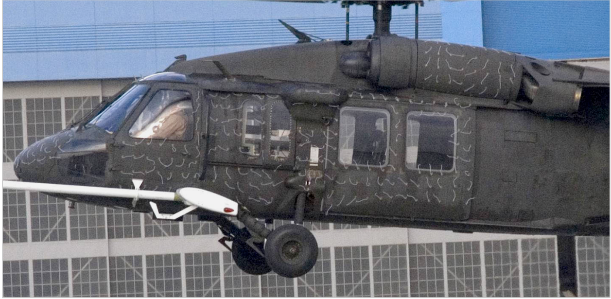
Figure 5(c). Single instantaneous airframe tuft pattern; Wheel height=5 ft.
