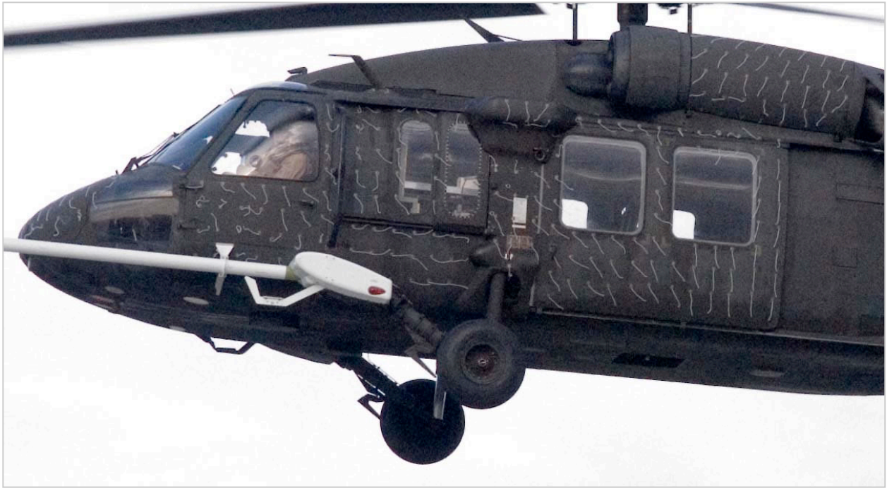
Figure 4(a). Single instantaneous airframe tuft pattern; Wheel height=50 ft.
