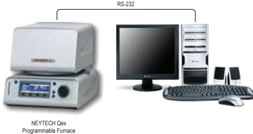
Figure 16. Furnace set-up designed and installed at AAMU.
