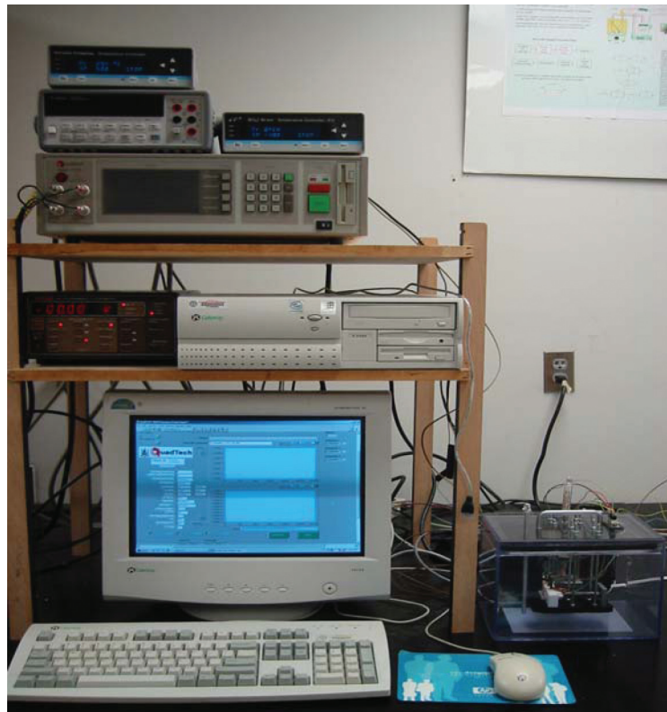
Figure 23. Photographic view of the set-up of the vapor testing station.
