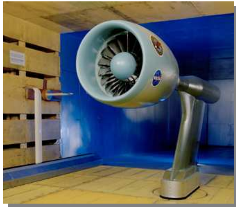
22" Advanced Ducted Propulsor in NASA Glenn 9'x15' Wind Tunnel
