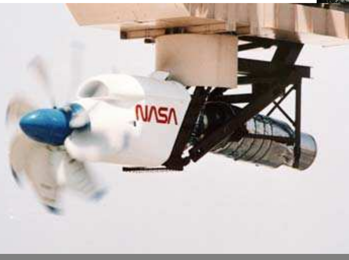
Large Advanced Propeller Full Scale Static Test
