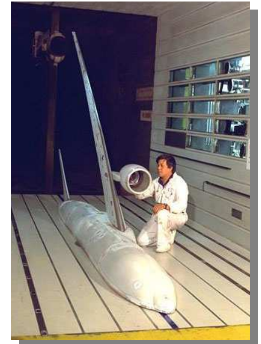
Propulsion/Airframe Integration Aerodynamics Test in NASA Ames 11' Wind Tunnel
