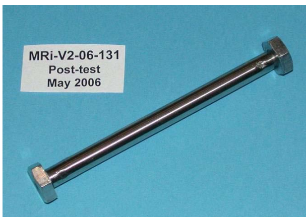
Fig. 7. Picture of a VPS formed NiTi shape memory tube for torque tube testing.
