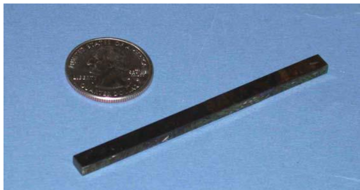
Fig. 5. Picture of a typical cantilever beam test specimen.
