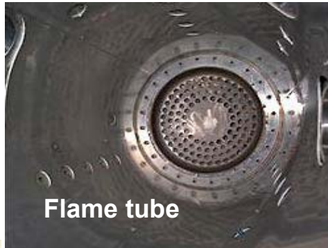
Low conductivity TBC flame tube and combustor deflector demos in Advanced Subsonic Combustion Rig (ASCR)
