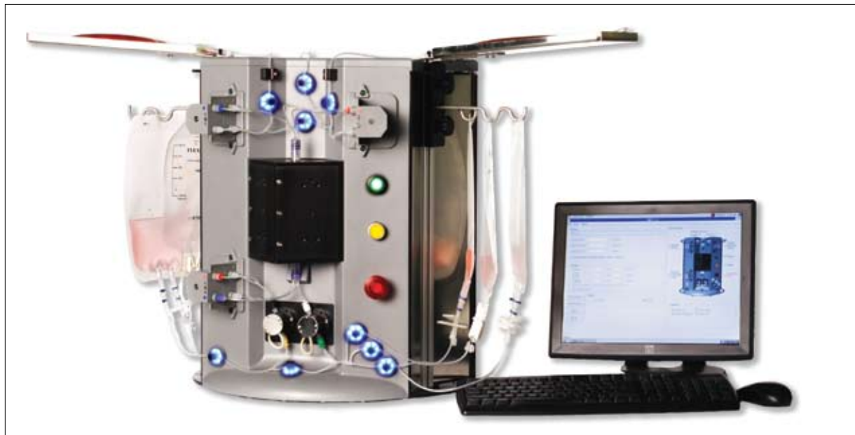
Techshot and IKOTech licensed and commercialized this Quadruple Magnetic Sorter, which uses magnetophoresis for cancer research and stem cell processes.
