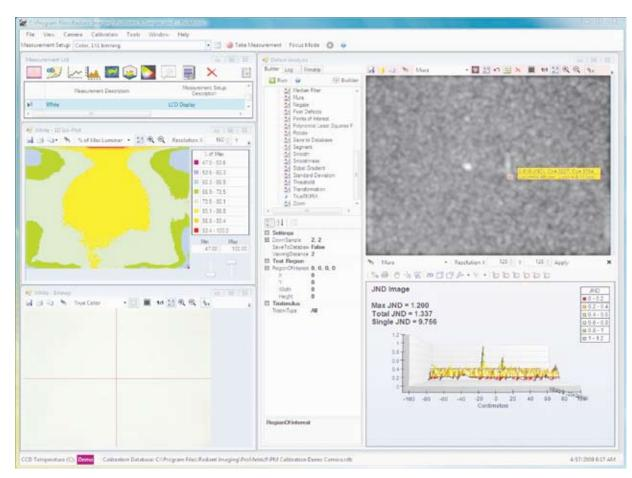
The Spatial Standard Observer is particularly useful for the inspection of displays during the manufacturing process.
