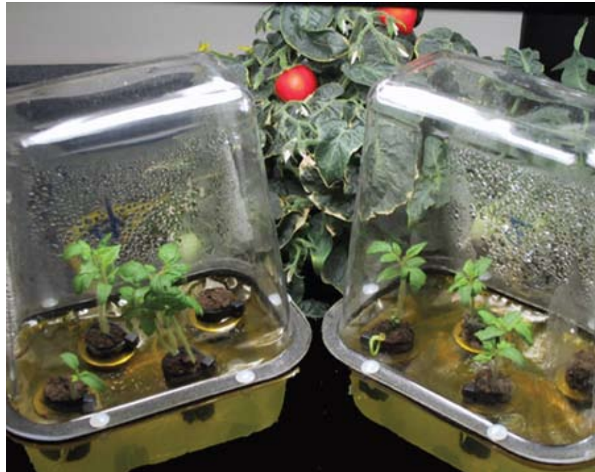
Tomato plants growing in the Plant Development Habitat (PDHab) at BioServe Space Technologies. For a recent experiment on the International Space Station, the PDHab was loaded into a Commercial Generic BioProcessing Apparatus, a temperature-controlled microgravity research platform that has hosted a variety of experiments on numerous space shuttle, Mir, and ISS missions.
