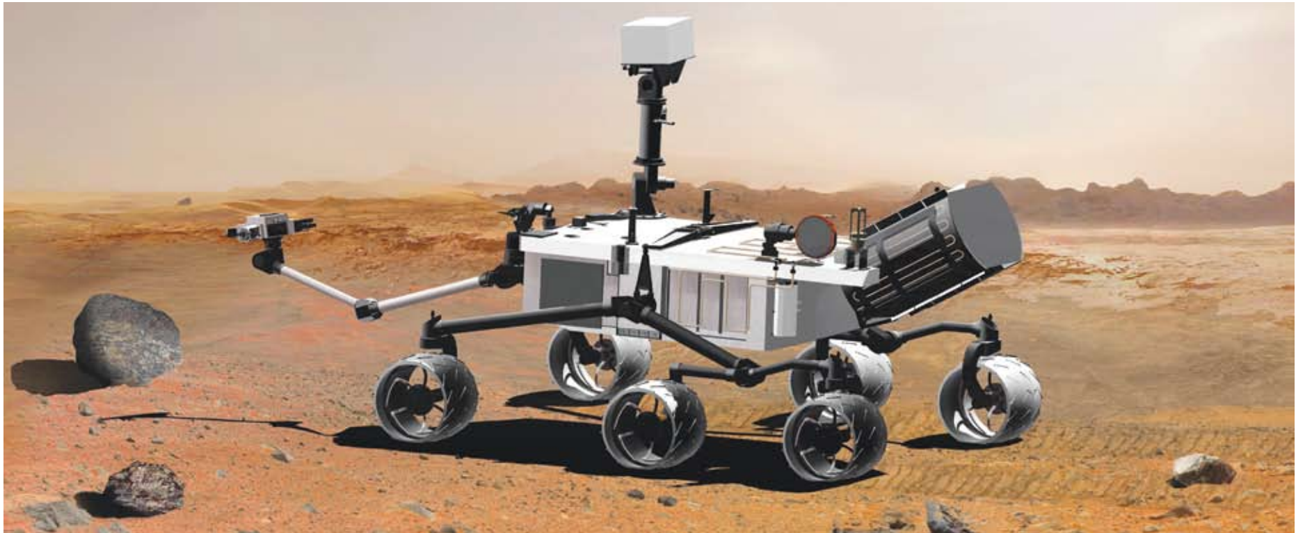
An artist's concept portraying NASA's Mars Science Laboratory, a mobile robot for investigating Mars' past or present ability to sustain microbial life. This picture is what the advanced rover, scheduled for launch in 2009, would look like in Martian terrain from a side aft angle. The mast, rising to about 2.1 meters (6.9 feet) above ground level, supports two remote-sensing instruments: the Mast Camera for stereo color viewing of surrounding terrain and material collected by the arm, and the ChemCam for analyzing the types of atoms in material that laser pulses have vaporized from rocks or soil targets up to about 9 meters (30 feet) away. The ChemCam incorporates the 3D Plus RTIMS.
