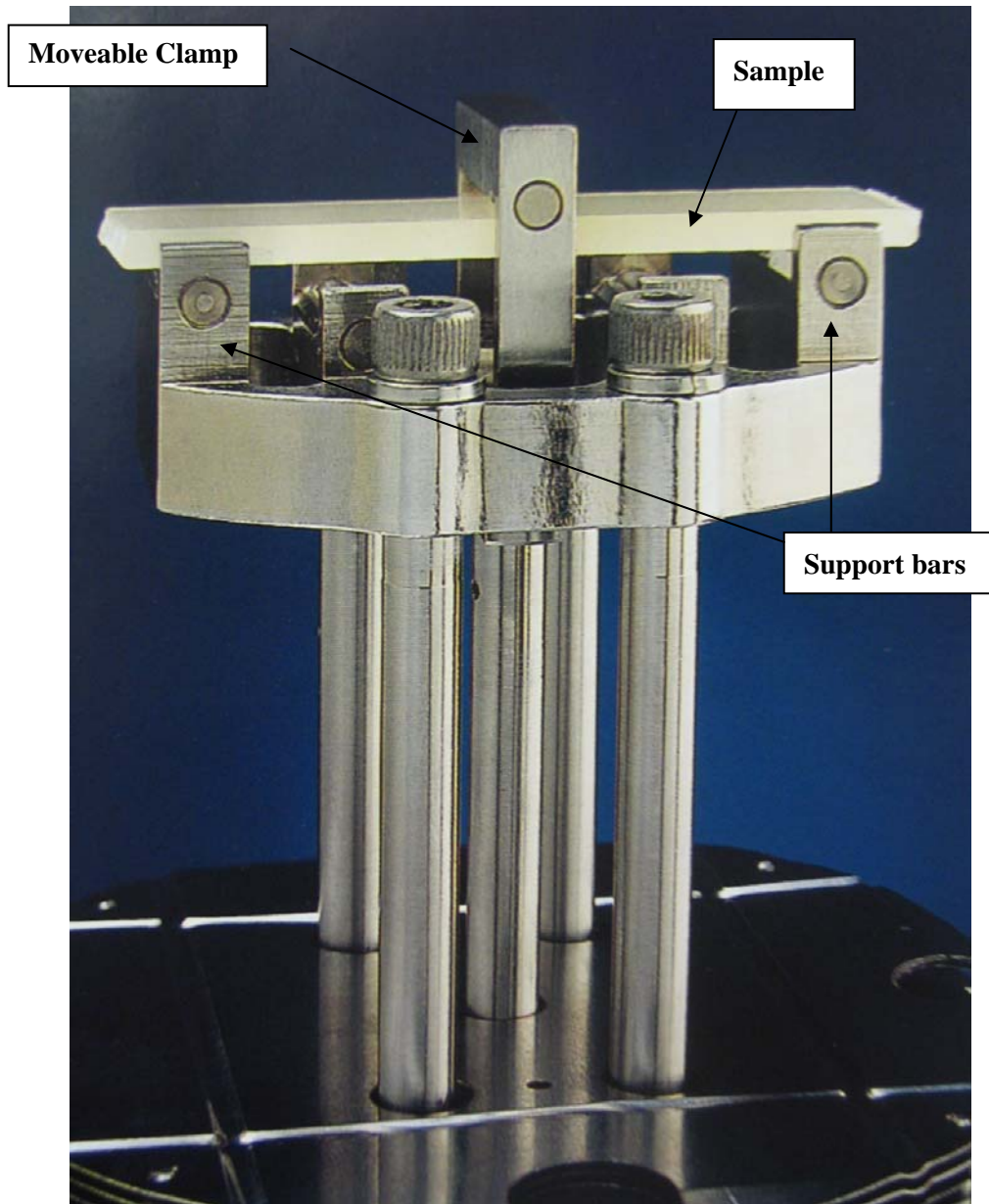
Figure 1. Dynamic Mechanical Analyzer with 3-Point Bend Clamp Installed
