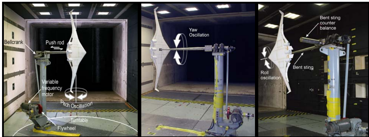
Fig. 13 Forced-Oscillation setup of 3% scale BWB model.
