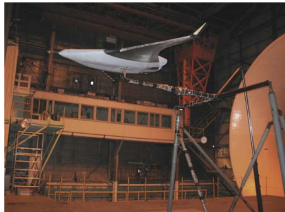
Fig. 18 Static force and moment test set-up of 5% scale model in LFST.
