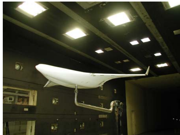
Fig. 11 BWB 3% scale model on bent sting mount.
