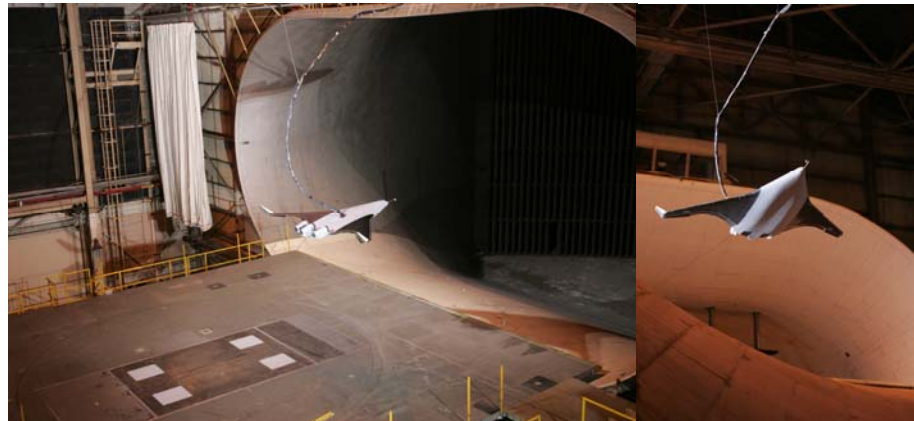
Fig. 15 BWB free-flight test in Langley Full-Scale Tunnel.
