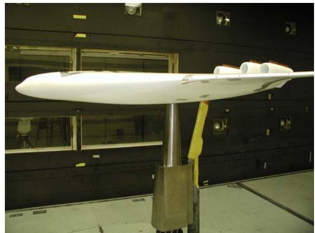
Fig. 7 BWB 3% scale model on post mount.
