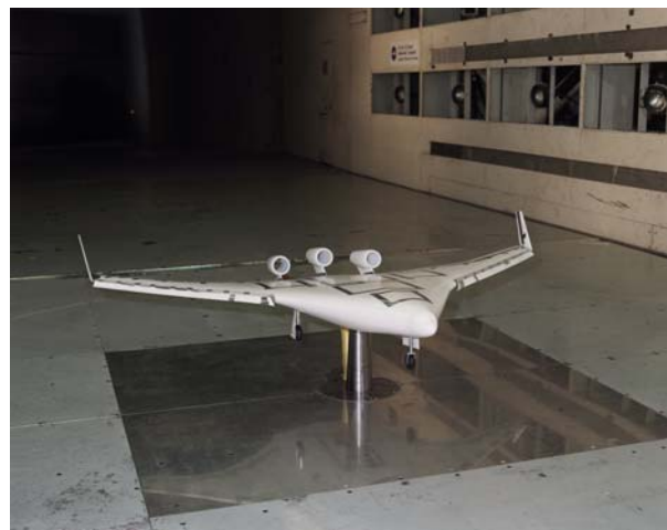
Fig. 8 Ground effects test on post mount.
