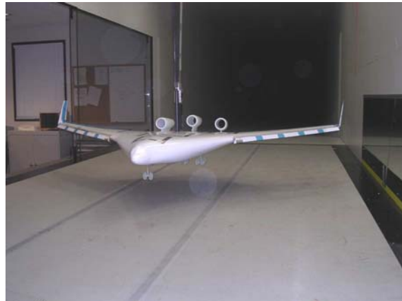
Fig. 14 Ground effects test of 3% scale model in Swift Engineering tunnel.
