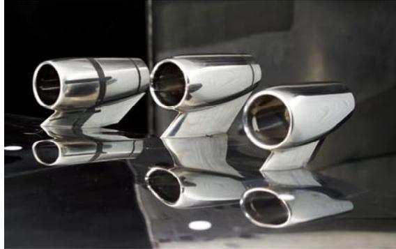
**Fig. 2 BWB model with boundary layer ingestion nacelles.**
