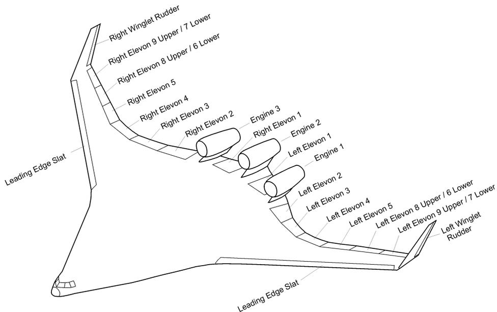
**Fig. 4 BWB full scale configuration control surfaces**
