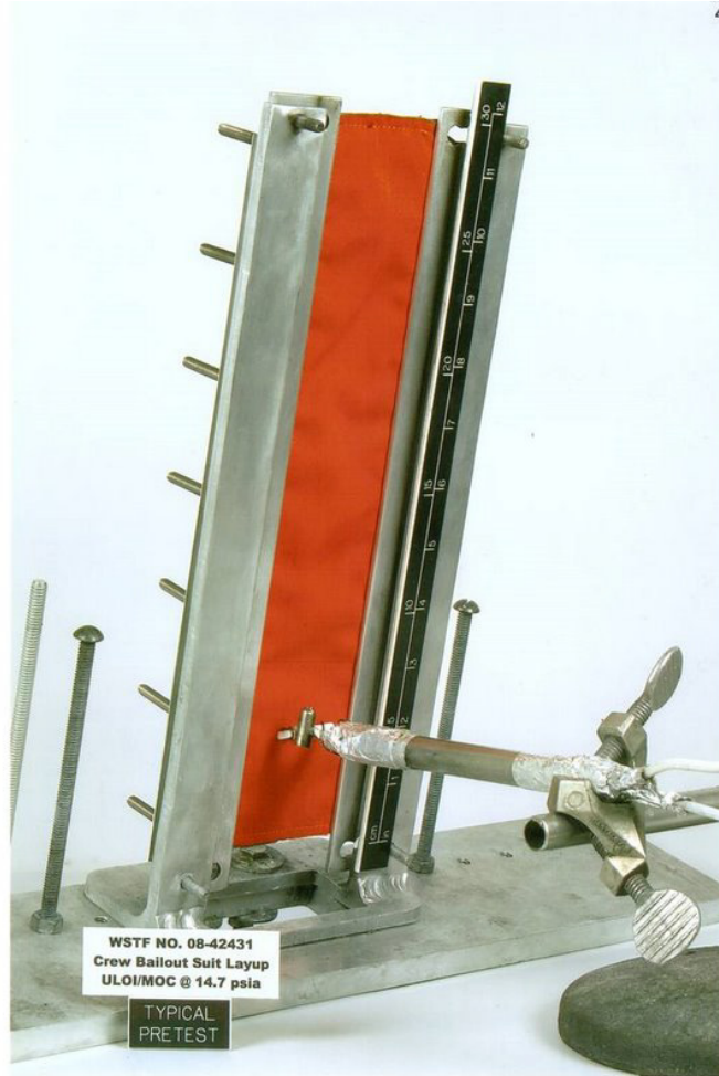
Material Flammability Testing
