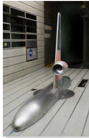
Half-span model test in Ames 11' wind tunnel
