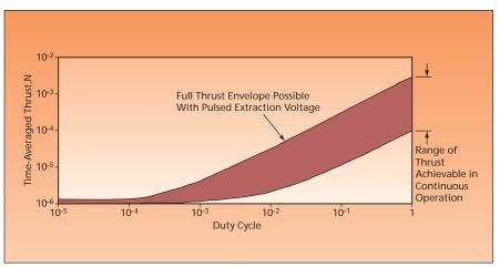
**Time-Averaged Thrust** was calculated theoretically for a representative ion thruster operating in continuous and pulse modes. A minimum average thrust much lower than that attainable in continuous operation (about 1  $\mu$ N, below which the thrust due to ion flux is comparable to the flow of the propellant gas without ionization) would be achieved by pulsing at a low duty cycle.
