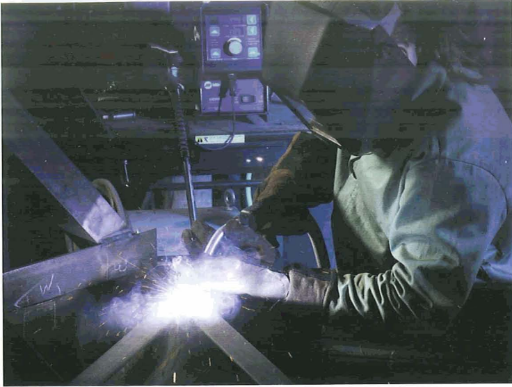
Bob Peters, of Kendel Welding and Fabrication, welds part of an internal access support for the Ares I-X upper stage simulator at NASA's Glenn Research Center in Cleveland. In 2009, NASA will launch Ares I-X, a test flight for the new Ares I rocket. Ares I will launch astronauts on missions to the space station, the moon and beyond. (21995main_image-eng)
