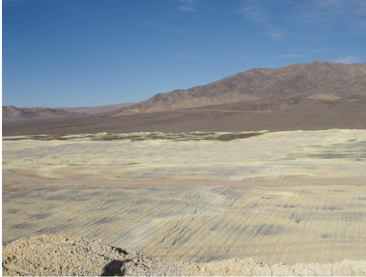
Figure 4: Copper bioleaching; heap and dump reactors in the Atacama Desert of northern Chile.
