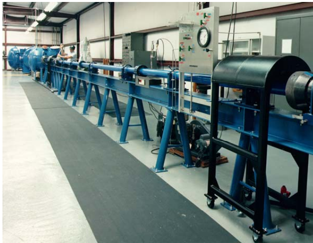
Figure 2-5. WSTF .50 caliber two-stage light-gas gun
