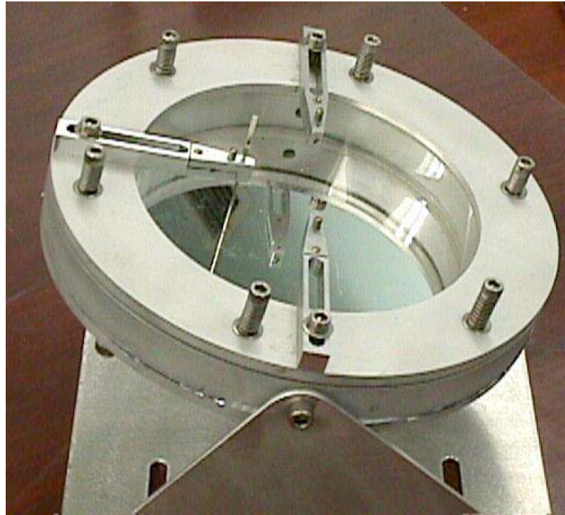
Figure 7-12. Test unit containing three sensors (one shown), for hypervelocity impact studies
