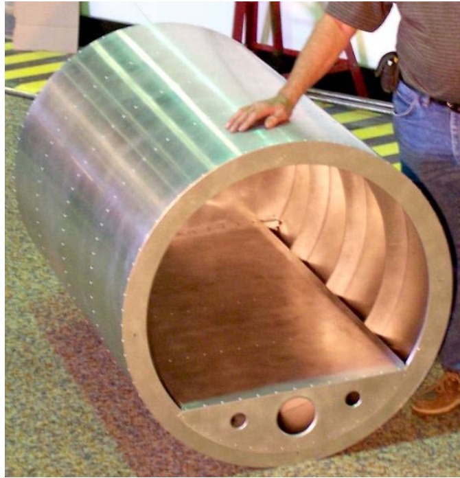
Figure 7-9. Small scale test structure designed to evaluate signal propagation
