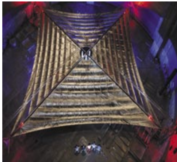
A solar sail of 20-meter edge length was successfully deployed in vacuum at the Space Power Facility at Plum Brook Station at the Glenn Research Center.
