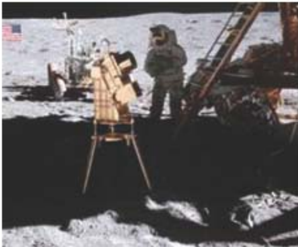
Apollo 16 far ultraviolet camera placed on the lunar surface by Astronaut John W. Young.
