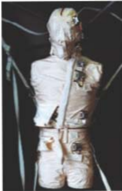
Photograph of Fred; a man-made model of a human torso flown on the ISS to measure typical radiation doses to internal human organs.
