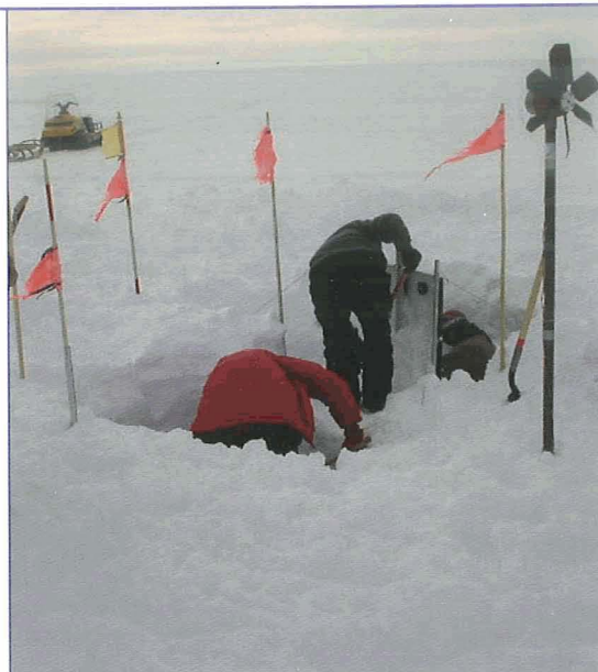
NASA Jet Propulsion Laboratory's team retrieving pressure and temperature sensors measuring the ice stream of the West Antarctic ice sheet.
