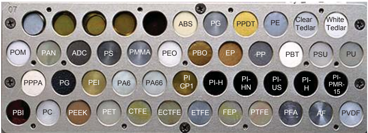
Figure 2.—Photograph of the MISSE 2 PEACE Polymers experiment prior to flight. The labels shown on the samples are defined in table 1.
