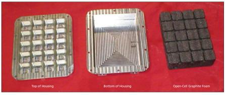
The Components Shown Separately here were assembled to make a heat-storage module. Prior to sealing the module, the open-cell graphite foam was filled with molten LiNO<sub>3</sub>·3H<sub>2</sub>O containing small proportions of a surfactant and a freezing catalyst.
