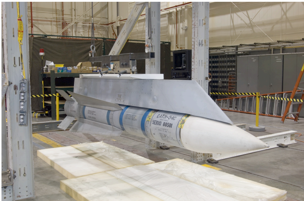
Figure 1. Weight and CG test setup.
