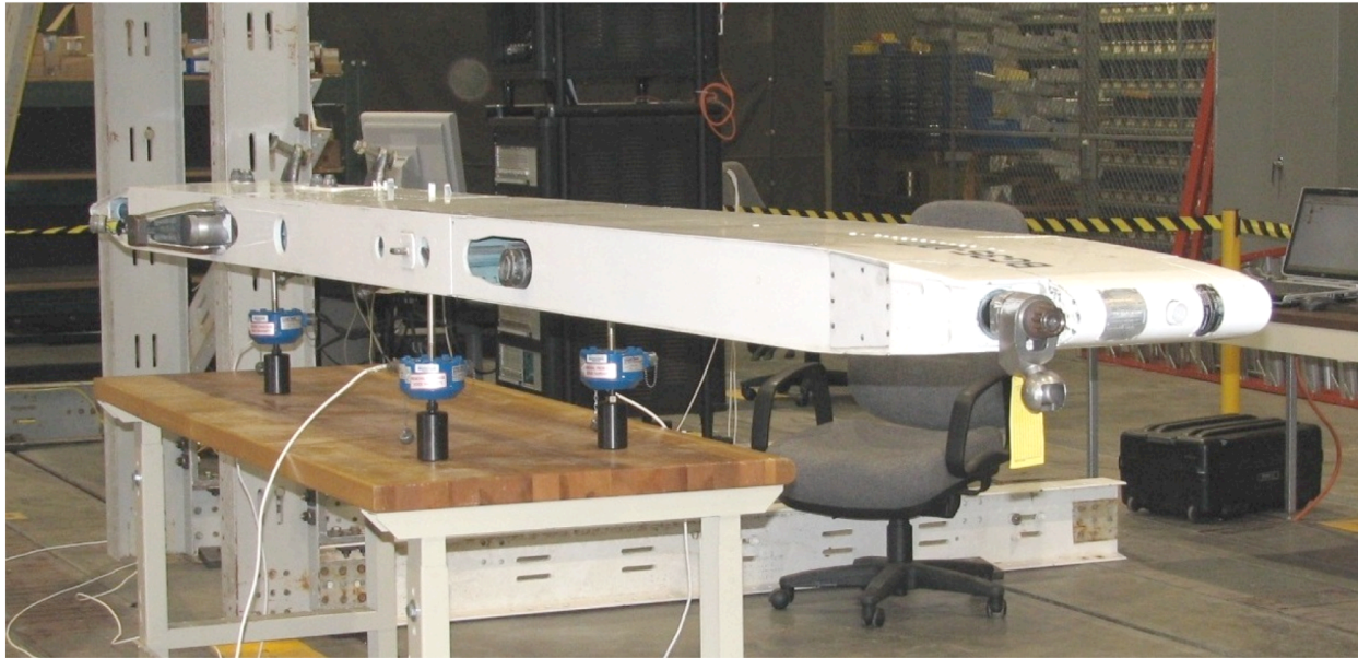
Figure 1. Weight and CG test setup.
