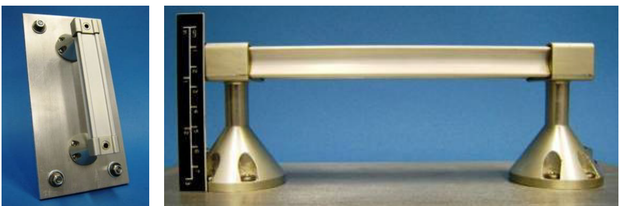
Figure 6: ISS tube handrail (P/N SDD33107728-073) subject to HVI testing in [5].
