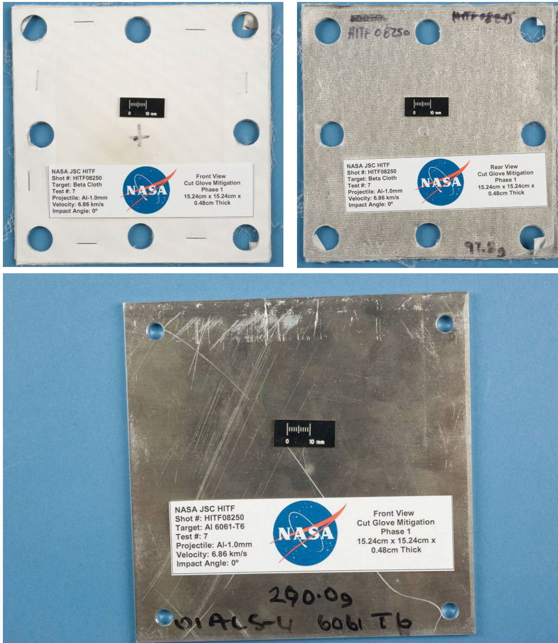
Figure 13: HITF08250 post-test damage photographs. Clockwise from top left: outer beta-cloth cover front side, innermost beta-cloth cover rear side, target plate front side.
