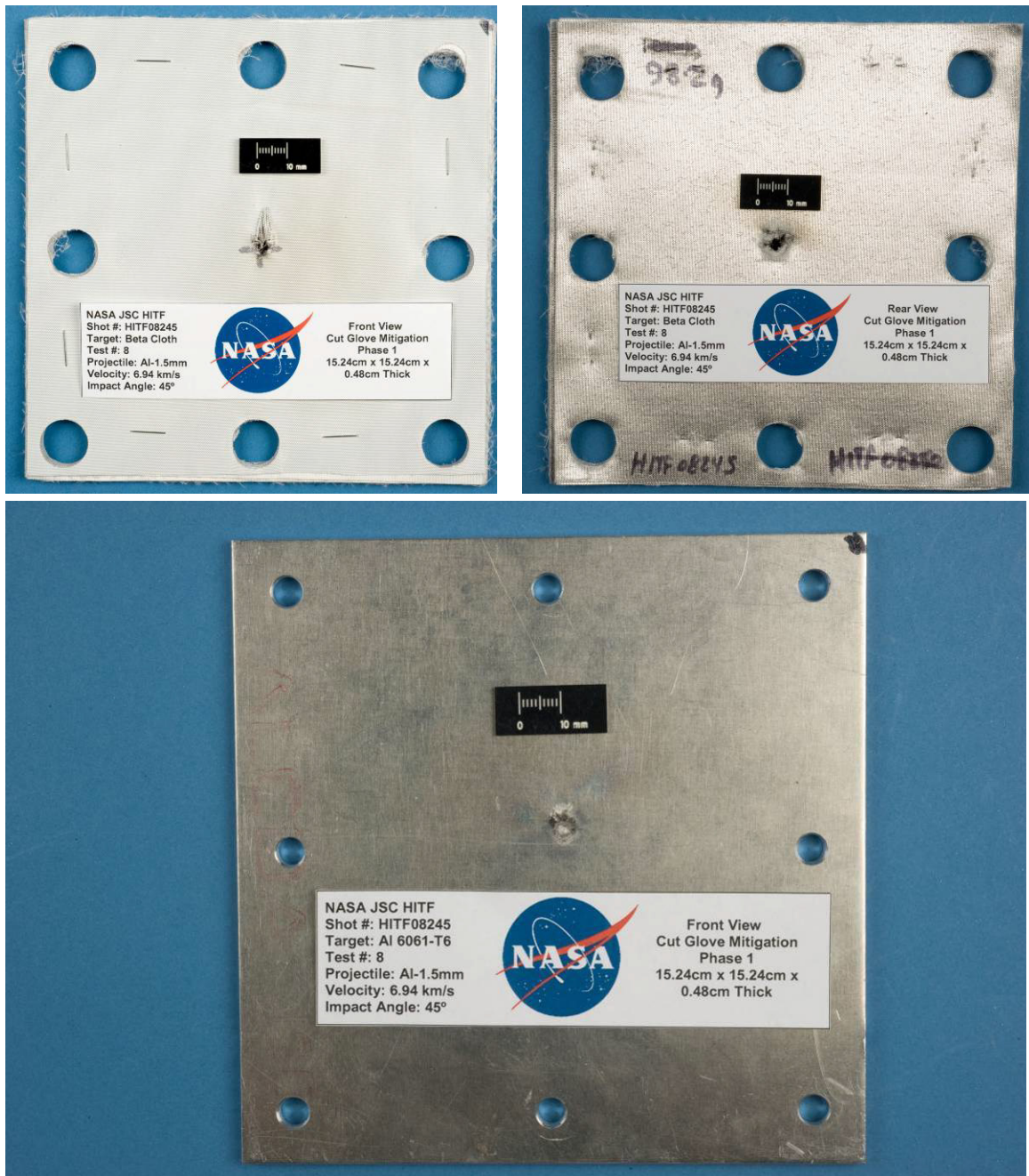
Figure 15: HITF08245 post-test damage photographs. Clockwise from top left: outer beta-cloth cover front side, innermost beta-cloth cover rear side, target plate front side.
