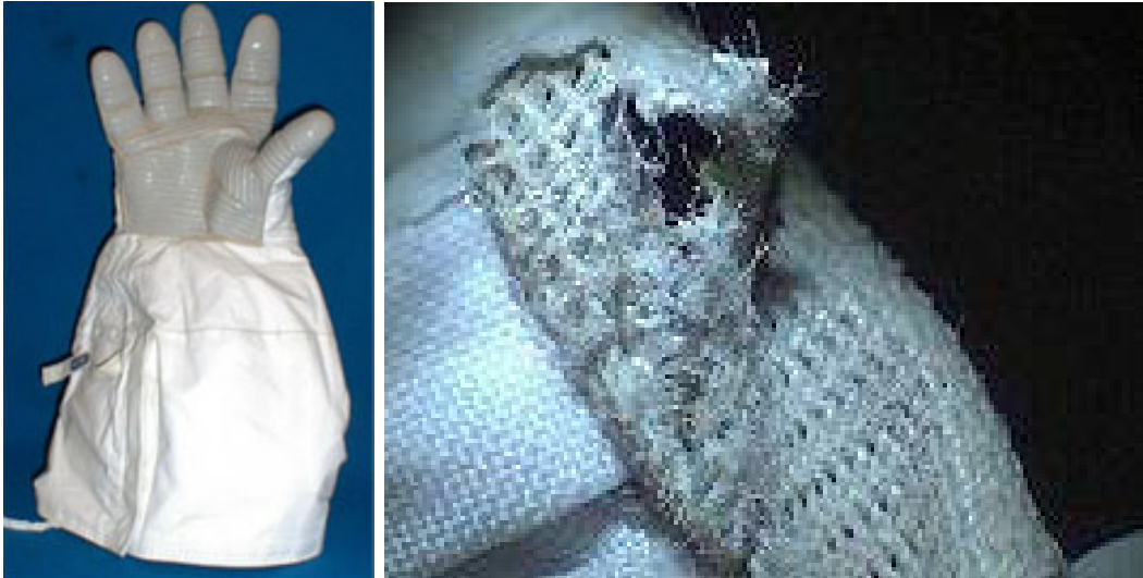
Figure 1: Damage to crewmember Curbeam's Phase VI glove following EVA 3 of STS-116.
