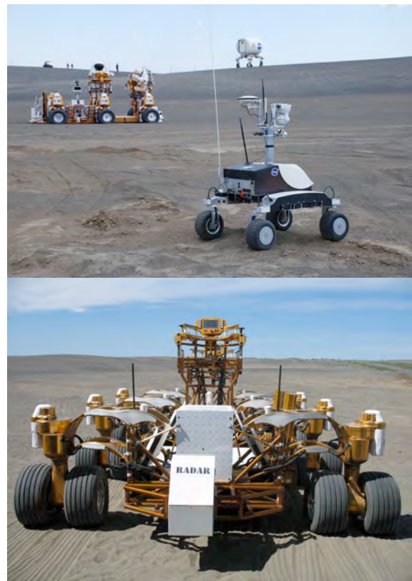
Fig 1: On the top in the front plan, K10 Black rover (NASA/AMES), performing subsurface reconnaissance in support of crew EVA (in the back plan). On the Bottom, the GPR mounted on the back-dock of the Chariot platform (NASA/JSC).
