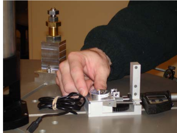
Assembling the shell supporting stage.
