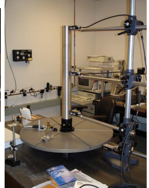
The non-contact displacement sensors are Keyence laser triangulation probes with a resolution of 10 nm and accuracy better than 60 nm.
