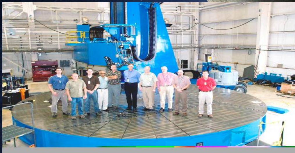
Robotic Weld Tool (RWT) MSFC Bldg 4755 gore-gore, dome-y ring, dome-fitting Self-Reacting Friction Stir Welding (FSW)
