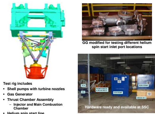
Figure 12. Helium Spin Start Test Rig and Test Hardware
