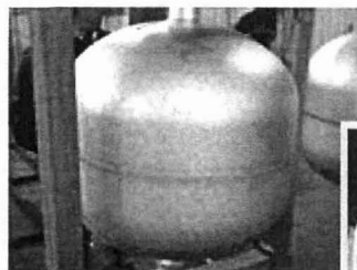
Chemically etched aluminum liner
