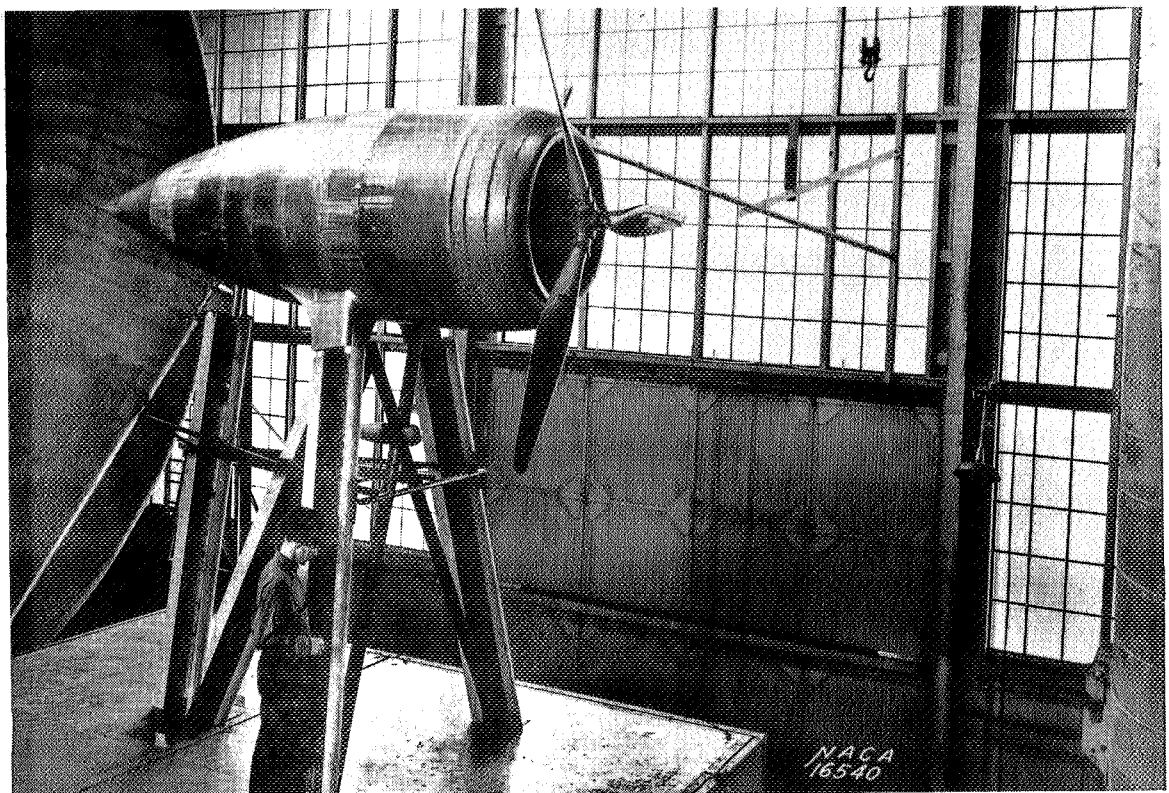
Figure 7.- Set-up 2, nose 1, nacelle 1 with a 1\frac{1}{2} -inch slot opening. The results discussed in this report were obtained with all slots closed and faired.
