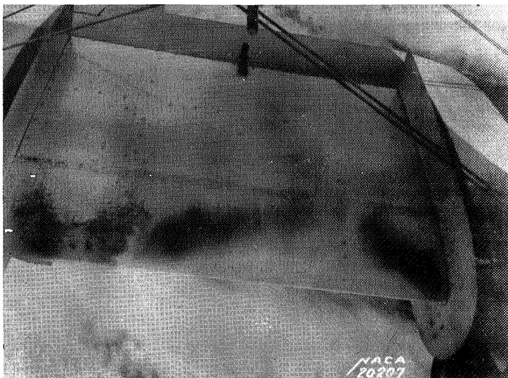
Figure 8.- Large pieces of ice being blown away less than 10 seconds after hot air was admitted to the wing
