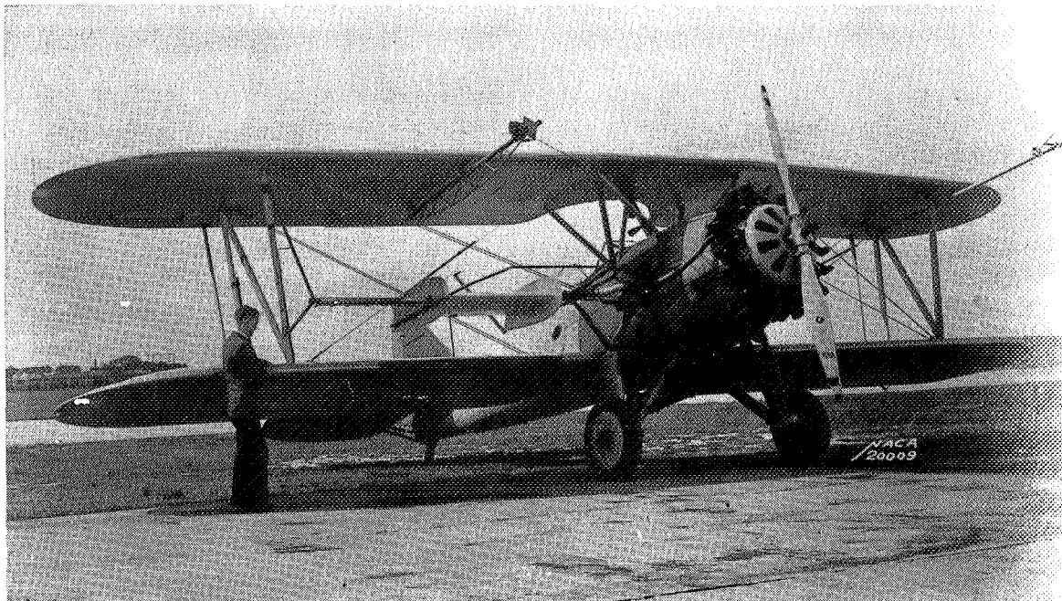
Figure 5(a).-- General view of XBM airplane, showing wing heated by hot air, and motion-picture camera mounted above and in front of the model wing.
