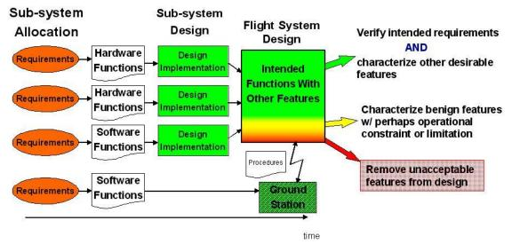
Figure 5.1-1. Flight System Development Process
