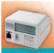
Del Mar DigiCorder Model 483 Holter Monitor, continuously records ECG of ambulatory subject. Image courtesy of NASA.
