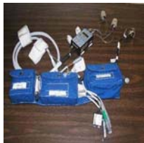
Continuous Blood Pressure Device (CBPD) is a non-invasive device that uses plethysmography to measure blood pressure at the finger. Image courtesy of NASA.
