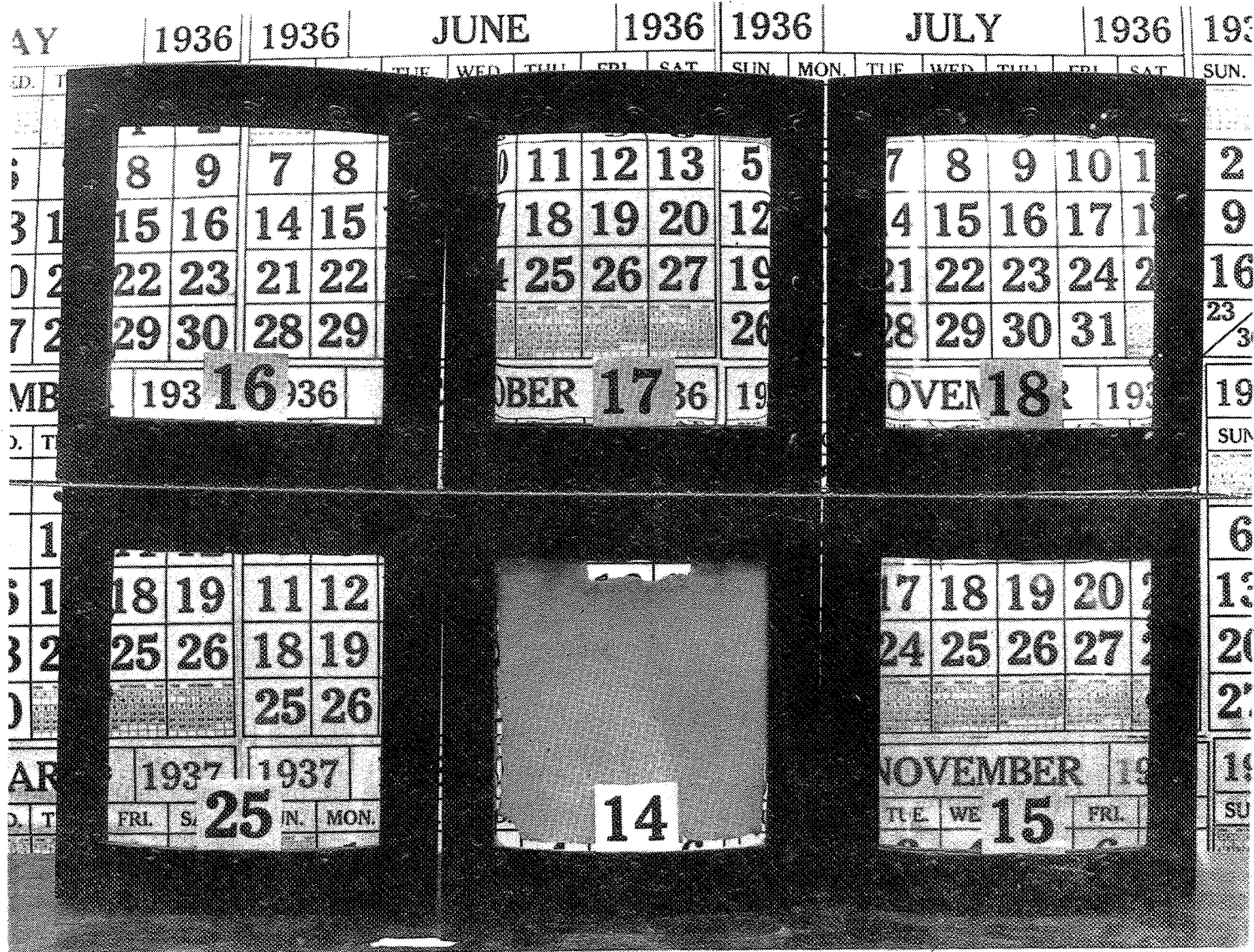
Figure 5.- Exposure panels after one year out-of-doors (sample 25 exposed for nine months only).
