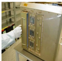
Lateral side view of MDS, with waste filter partially removed. Image courtesy of ASI.
