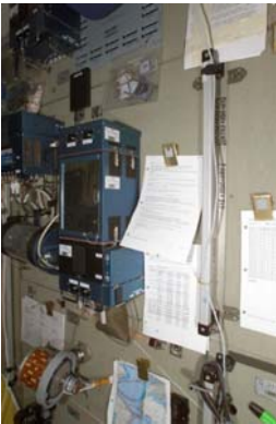
NASA Image: ISS006E27426 - View of Lada Leaf Chamber and Light Module on panel 218 in the Service Module, Zvezda during ISS Expedition 6. The Lada Greenhouse is used for growing vegetables in the Zvezda module of the ISS.
