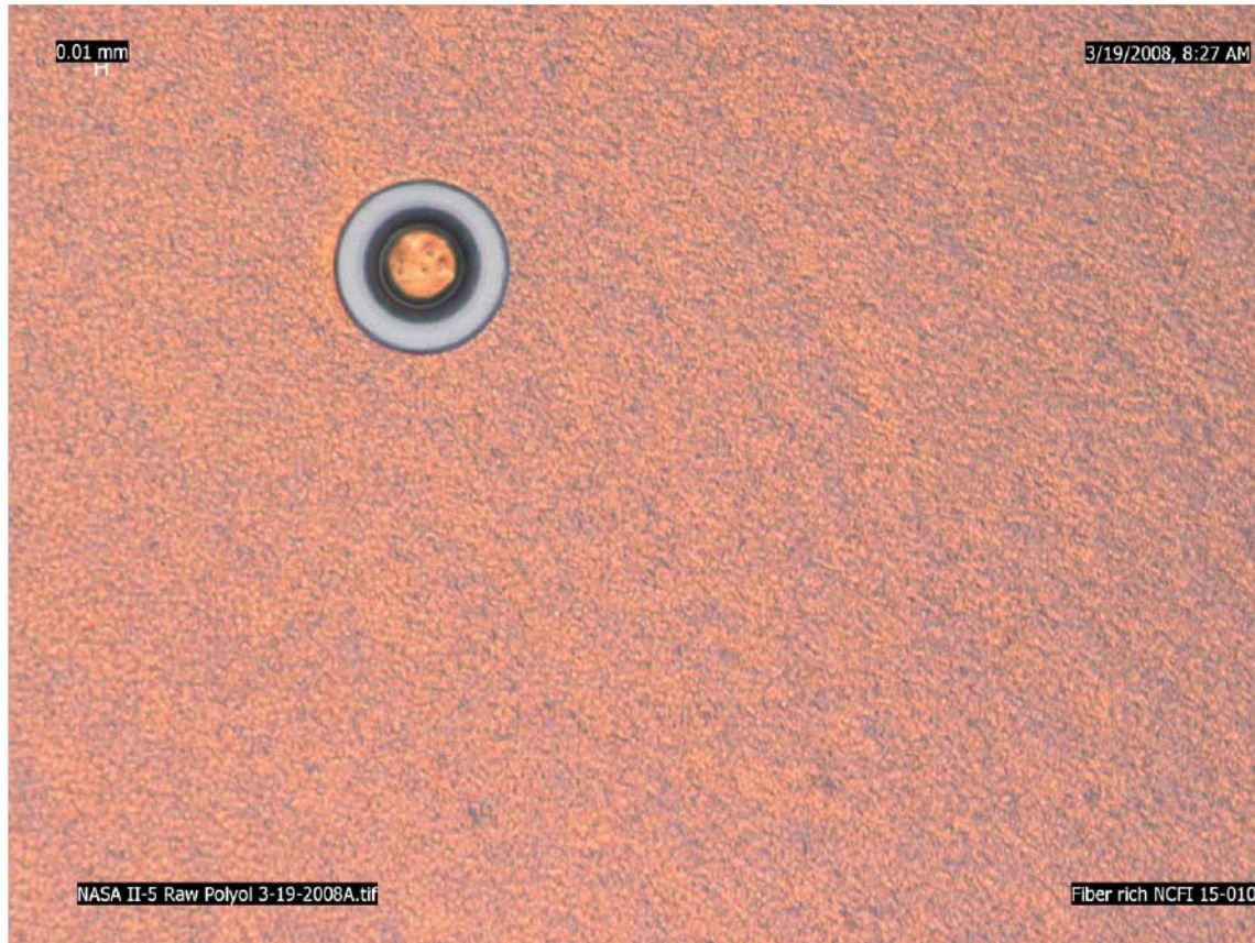
Figure 6 – NASA II-5 Raw Polyol and Milled Kevlar® Pulp (Note the tiny dark spots of fiber as opposed to larger scale fibrils in Figure 5)
