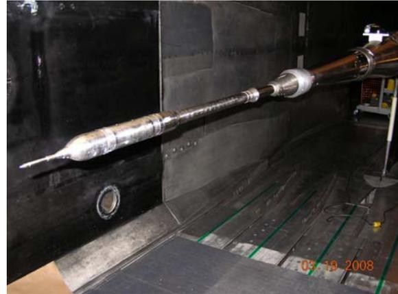
**Figure 7.** 1% scale pressure model inside the wind tunnel.
