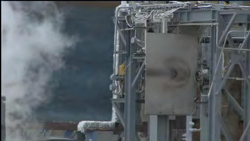
J-2X Workhorse Gas Generator Test Firing
