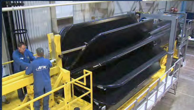
First Stage Fin Installation and Removal Testing
