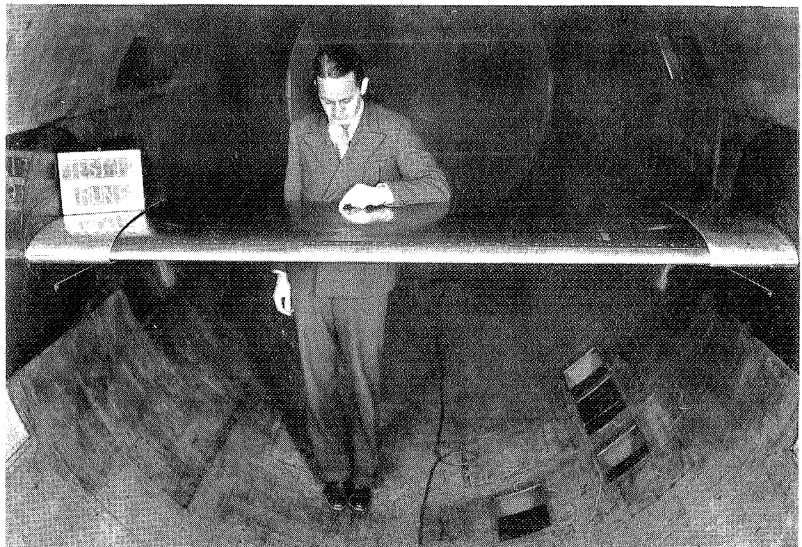
Figure 2.- The airfoil of 2-foot chord with 10 rows of rivets mounted in wind tunnel.
