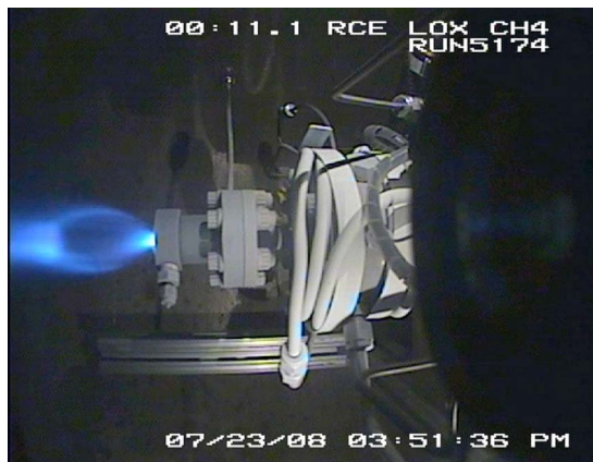
Figure 7.—Ignition test with nozzle at reduced igniter body temperature.
