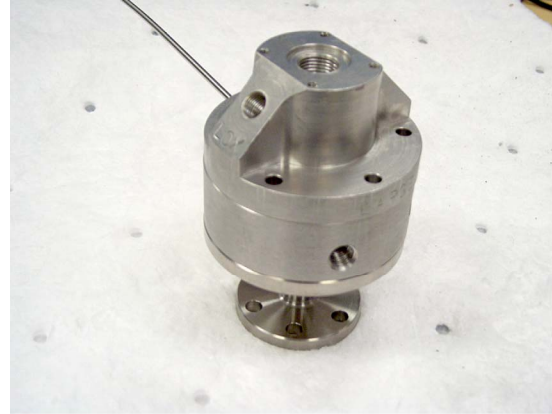
Figure 3.—Assembled igniter stack, chamber with center flame tube and pressure port attached, and coolant sleeve.
