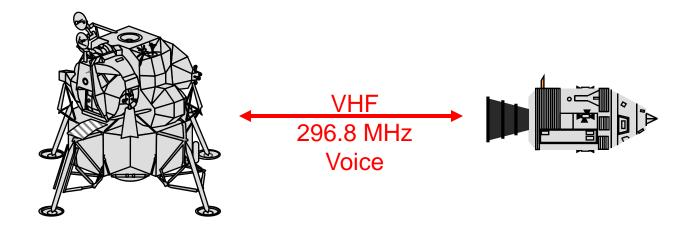
Simplex Operations = Transmit and Receive on the same frequency
