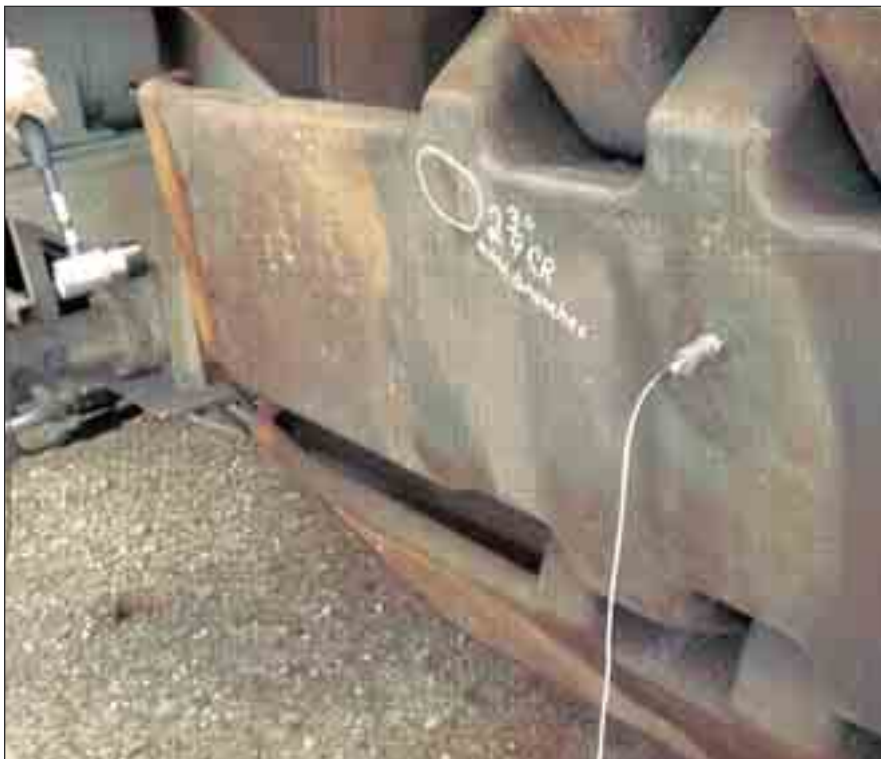
The Setup for Experimental MVA on a massive crawler tread shoe is simple and can be implemented easily: The placements of the modal-hammer blow and accelerometer are not critical.
