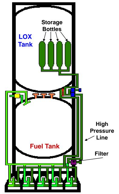
Four high pressure He Storage Bottles in LOX Storage Tank pressurized Fuel **Bottles** Tank ullage LOX Tank □ High Pressure Line used for filling Storage Bottles Vent and Relief Dump Valve Valve Filter in He fill line prevented contaminants from entering Flight Pressurization System Dump Valve for High Pressure emergencies Line **Fuel Tank** Filter
