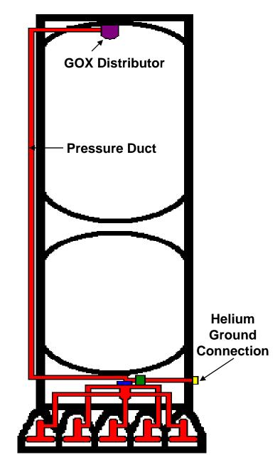
GOX was added to LOX Tank for pressurization during flight
